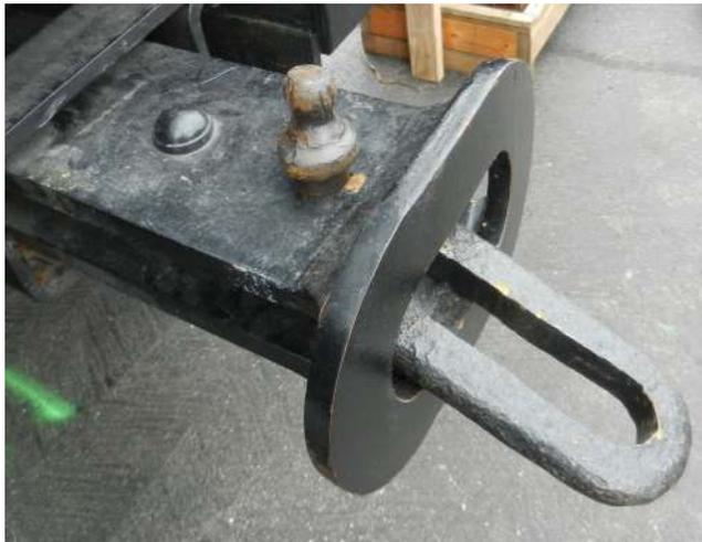
Figure 3. Example of a Link-and-Pin Coupling.
